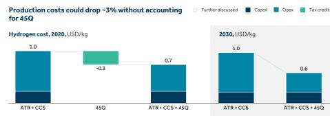
Plant capacity = 500,000 Nm<sup>3</sup>/h; natural gas = ~ \$2.5-3/MMBtu; greenbuild
